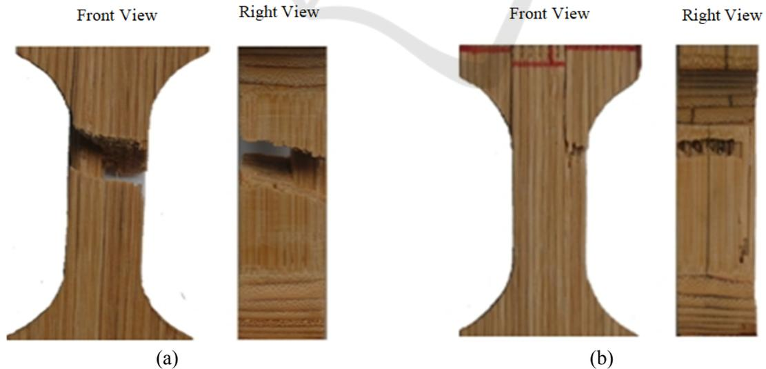
Figure 6. The failure mode of the laminated bamboo lumber under cyclic tension-compression loading ( $R=-1$ ): (a) in low-cyclic fatigue ( $N_f=1043$ ); (b) in high-cyclic fatigue ( $N_f=126020$ ).
