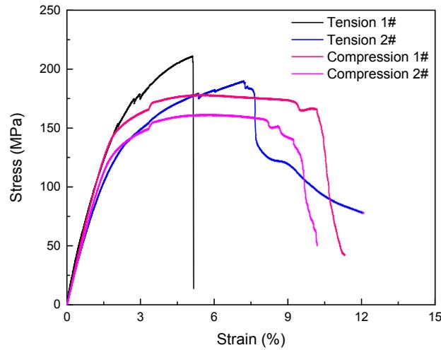
**Figure 3.** Stress-strain curves under tension and compression loading.
