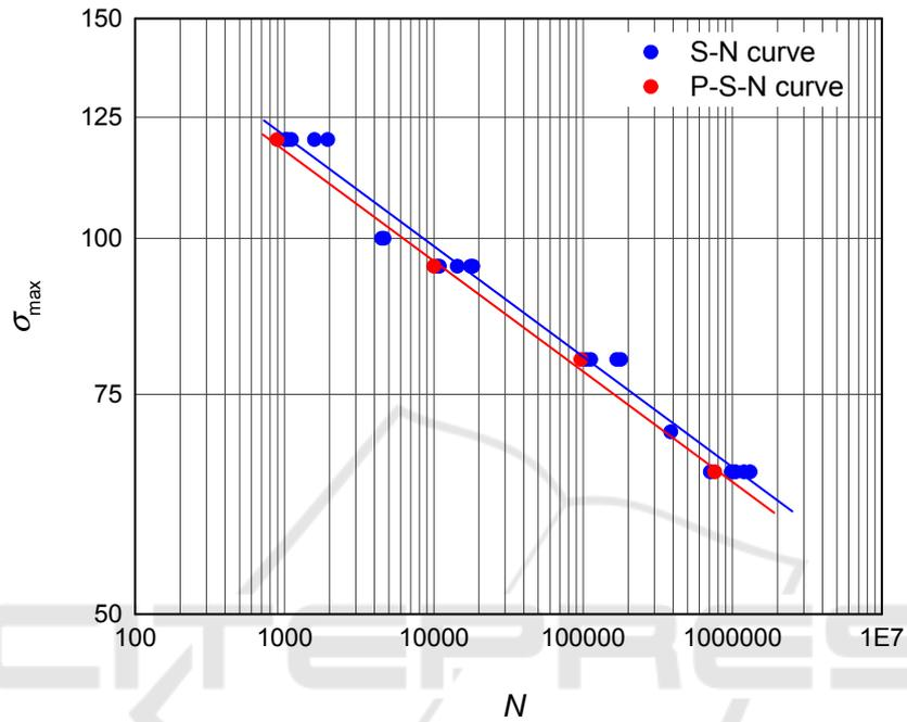
Figure 5. Stress-life curve for bamboo-based composites at  $R=-1$ .
