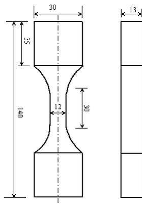
**Figure 1.** Details of the specimen geometry.
