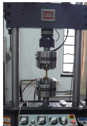
**Figure 2.** Specimen installed in fatigue machine..
