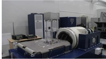
**Figure 10.** Sinusoidal sweep vibration test.
