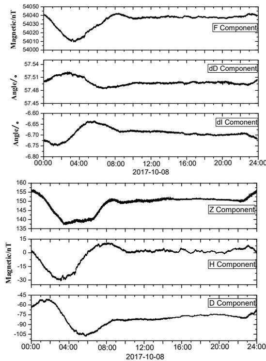
Figure 4: The geomagnetic diurnal variation curve of two developed sensor on Jinghai observatory(upper is dIdD, down is fluxgate sensor ).
