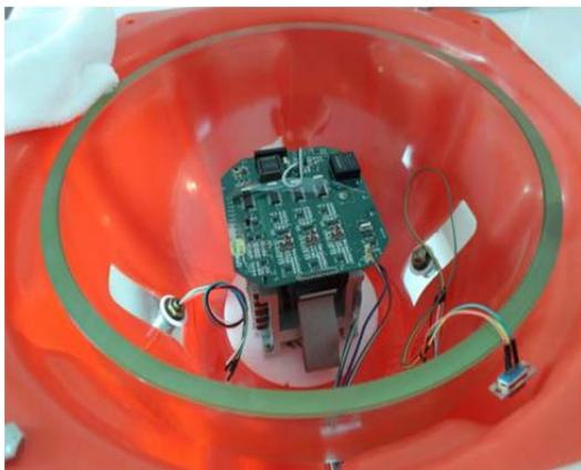
Figure 2: The developed fluxgate sensor (left is structure schematic, right is physical photo)
