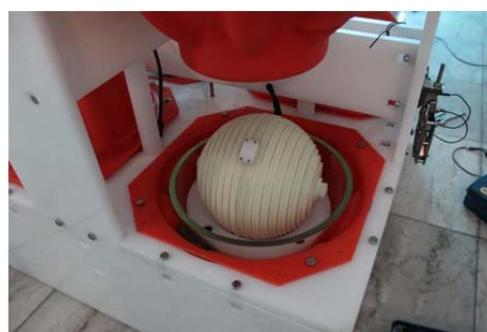
Figure 1: The developed dIdD sensor (left is structure schematic, right is physical photo)
