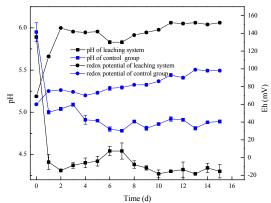
Figure 4: The pH and redox potential of leaching desulfurization test.
