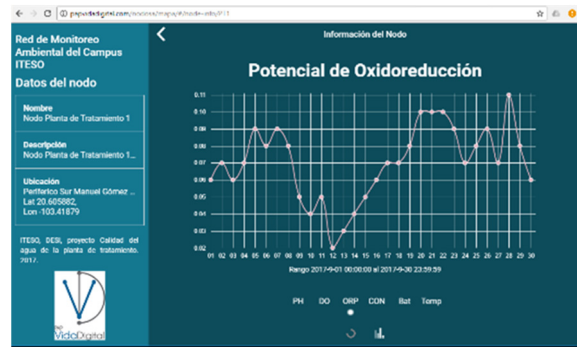
Figure 9: Example of webpage showing Oxydation Reduction Potential values of water.
