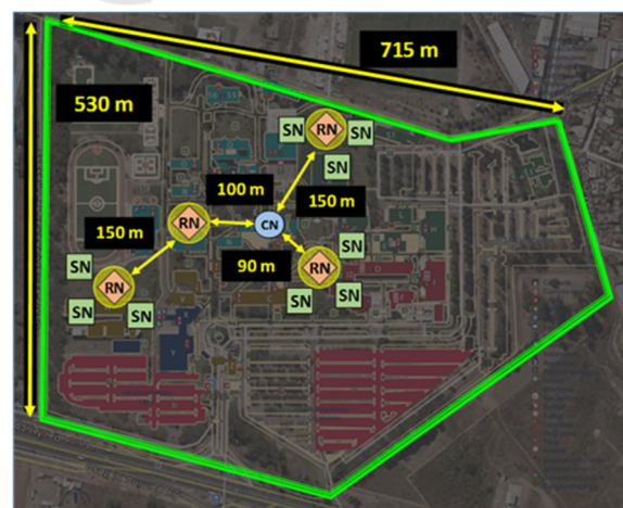
Figure 8: The Wireless Sensor Network Architecture.
