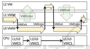
Figure 4: Flow of execution in a nested virtualization setup ("Unsafe Nested Virtualization on Intel CPU", 2018).
