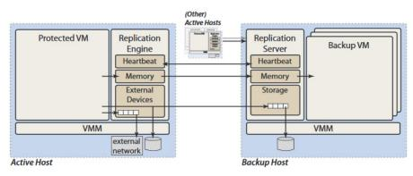
Figure 6: Remus high-level architecture (Cully et al., 2008).
