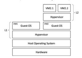
Figure 3: Nested virtualization setup (Berghmans, 2010).
