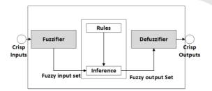
Figure 1: The overall representation of the functioning of a fuzzy system.
