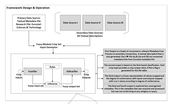
Figure 2: The Framework Design, Operation and perceived system outputs are described in this picture. It represents the functionality of the designed and attributed system for analysing textual metadata.
