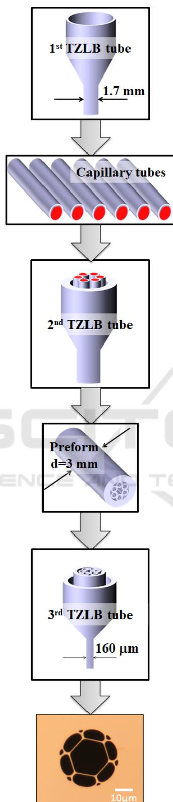
Figure 3: Schematic and experimental images of the fabrication of a TZLB HC-PCF.
