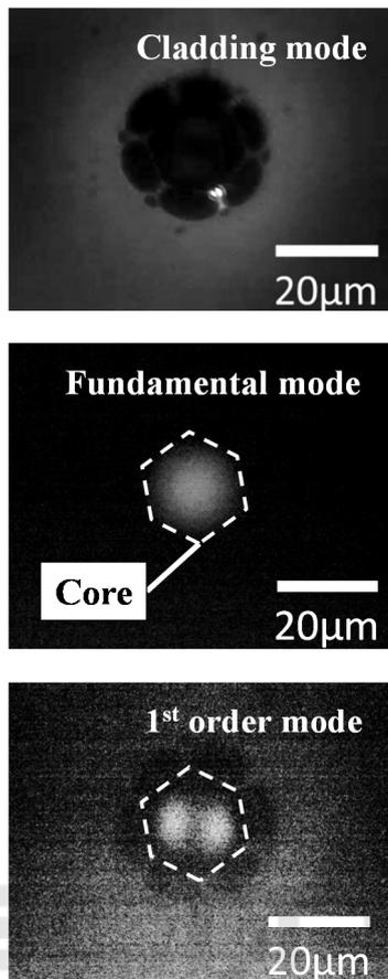
Figure 5: Images of different modes which were able to propagate in the tellurite HC-PCF.
