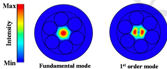
Figure 6: Calculated results of modes which can be confined in a tellurite HC-PCF.
