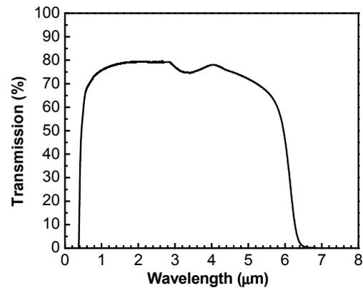
Figure 1: Transmission spectrum of the TZLB glass.
