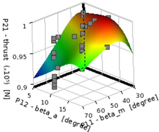
Figure 7: The response surface in assessing the effect of  $\beta_a$  and  $\beta_m$  on the thrust.
