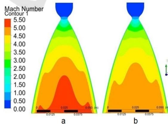
Figure 4: The Mach number distribution along the length of the chamber when using: a – single global reaction; b – set of 18 reactions.
