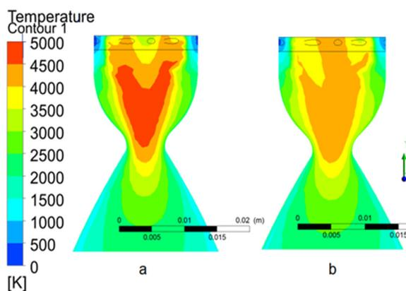
Figure 3: The temperature distribution along the length of the chamber when using: a – single global reaction; b – set of 18 reactions.
