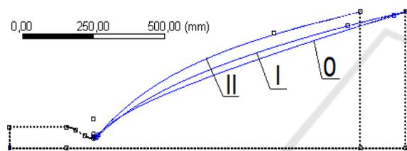
Figure 8: Changes the nozzle shape in comparison with the basic version ("0").
