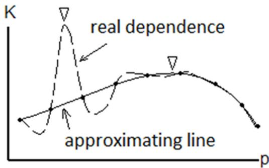
Figure 2: Error estimating the global maximum of the optimized criterion in the case of insufficient discretization of the approximation domain.
