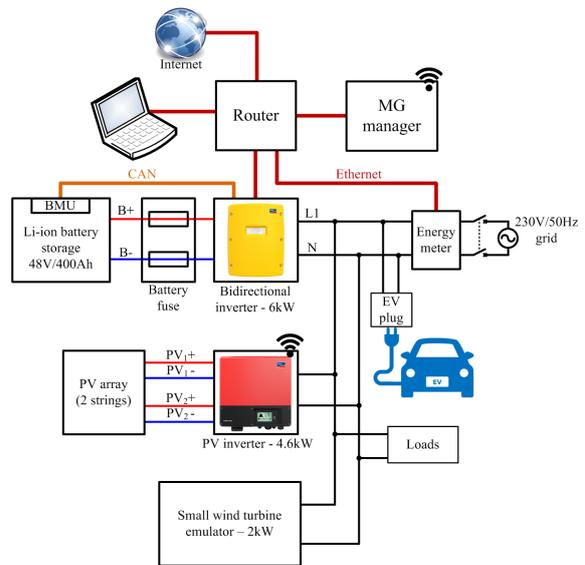
Figure 4: Diagram of the MG charging station for EVs.
