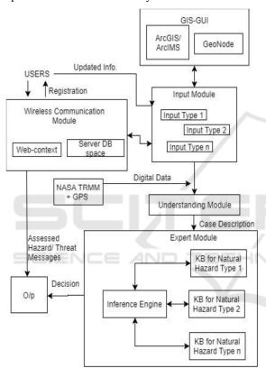
Figure 1: Schema SmaCiSENS modular architecture & data flow
