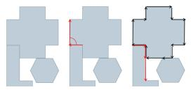
Figure 6: Algorithm to search for room polygons.
