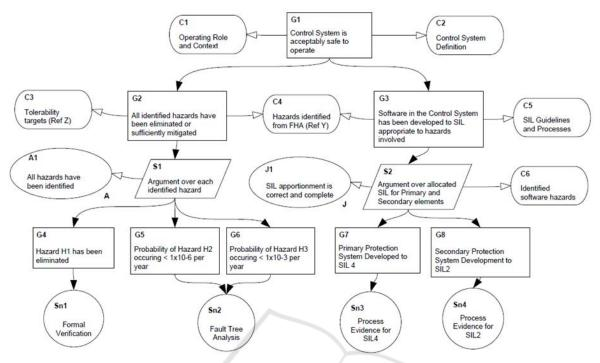
Figure 1: Example of GSN diagram (Goal Structuring Notation, 2017).
