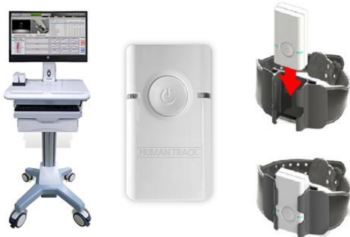
Figure 2: Hardware design of the IMU (the sensor was placed in the holder).
