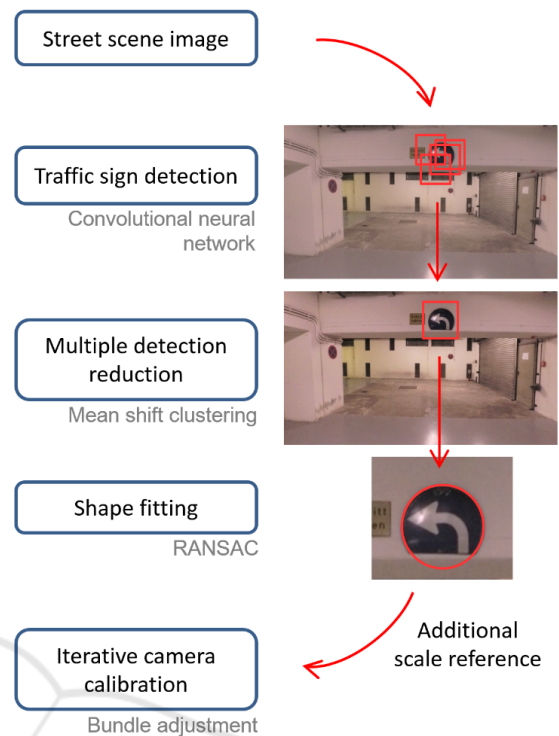
Figure 2: Processing steps performed for one iteration of the iterative camera calibration. Input is a street scene image recorded by a vehicle camera, whereof additional scale references for the camera calibration are extracted. Output are new estimates for the intrinsic parameters obtained by bundle adjustment. A new iteration of these steps is performed for each image captured over time when the vehicle is on the road.
