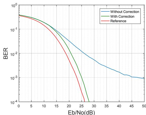
Figure 9: BER with and without correction and comparison with the reference case (no SFO) in the aircraft PLC channel 1.
