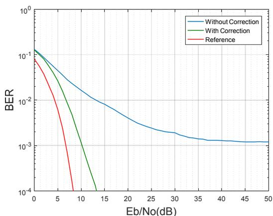
Figure 4: BER with and without correction and comparison with the reference case (no SFO).
