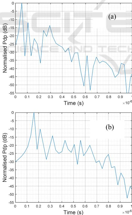
Figure 8: Channel impulse response for channel 1 (curve a) and 3 (curve b), the highest peak being normalized to 0 dB.
