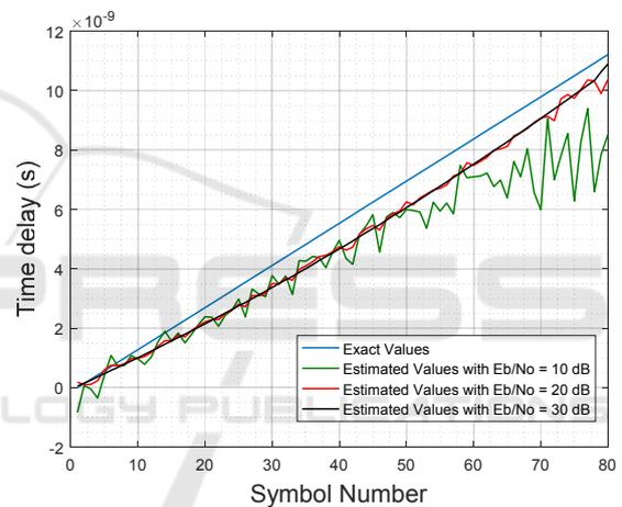
Figure 3: Performance of the estimator with 10 ppm offset.
