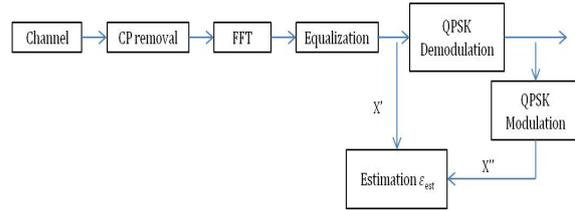
Figure 1: Blind estimation process at the receiver.
