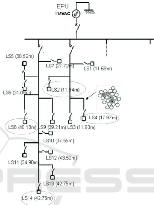
Figure 6: Geometrical architecture of a sub network of a cabin lighting system.
