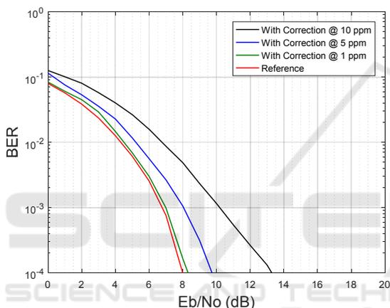
Figure 5: BER calculated in presence of an SFO equal to 1,5 and 10 ppm and comparison with the case of perfectly synchronized clocks.
