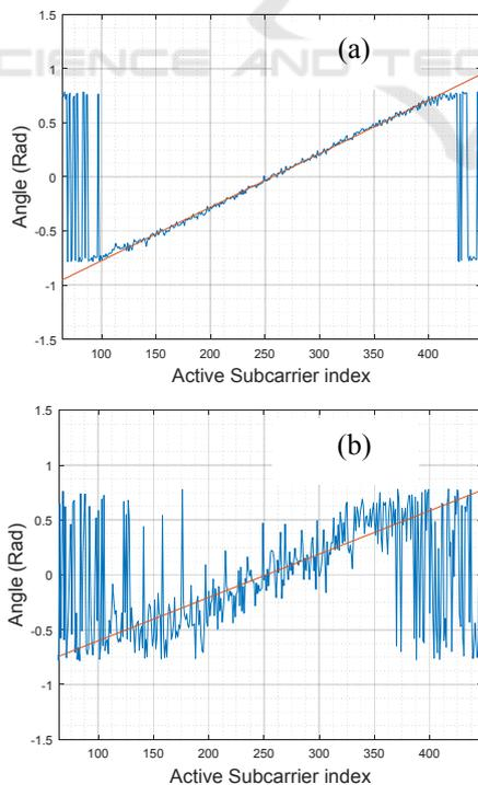
Figure 2: Phase variation versus the subcarrier index. (a)  $E_b/N_0 = 10$  dB, (b)  $E_b/N_0 = 30$  dB.
