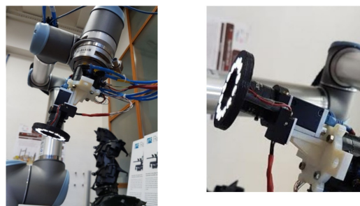
Figure 5: The industrial camera with a light ring mounted on the UR-10 robot with the pneumatic tool changer system. Left: a general view. Right: a close-up view.
