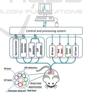
Figure 2: Scheme of the diagnostic system.
