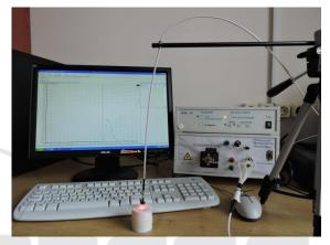
Figure 1: Diagnostic system "LAKK-M".
