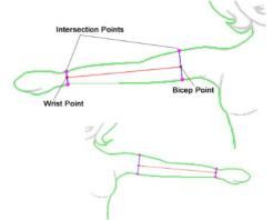
Figure 3: Skin-skeleton mapping of arm points. The system extends a line (red) from the bicep to the wrist, forming the arm axis. It then extends lines (blue) perpendicular to the arm axis, towards the outline, and looks for the intersection points (purple) with the skin. Finally, bicep and wrist points are centered between the two purple intersection points.
