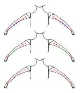
Figure 4: Limb Axis Correction Process. Top: some midpoints (blue) have intersection points (purple) from one side only because of unfitted axes. Middle: using single-sided intersections, the system extends perpendicular lines (green) towards the opposite side to
