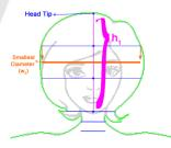
Figure 5: Head Dimensions. For  $1^{\text{st}}$  approach: h1 is the length of *l*, the line between the head tip and the neck top point. For  $2^{\text{nd}}$  approach: w2 is the smallest diameter found in the middle section of the head.
