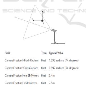
Figure 2: Field of view of the Positional Tracking Camera of the Oculus Rift.
