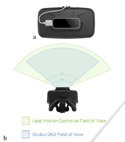
Figure 1: (a) Leap Motion device mounted on the Oculus Rift DK2 (b) FOV of the Oculus Rift and of the Leap Motion device.
