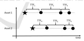
Figure 1: Collecting Times to Failure TTFs.
