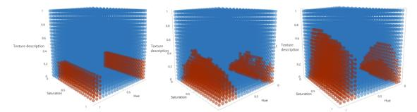
Figure 9: Classification of each of the methods for a set of points normalized from 0 to 1 of the 3 characteristics. First is the decision Tree, then KNN and finally SVM.
