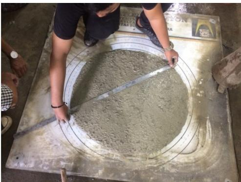
Figure 2: Slump flow test
