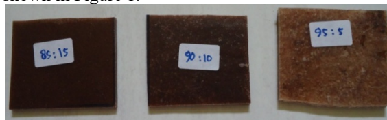
Figure 1. Specimen of respective WPC for durability testing in various proportions of plastics and wood filler (85:15, 90:10, and 95:5)
