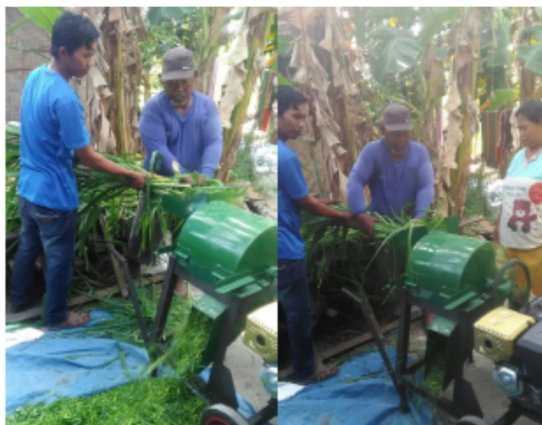
Figure 3. The farmer and rancher practiced the chopper machine to reduce size of paddy straw before make a fertilizer and animal feed.
