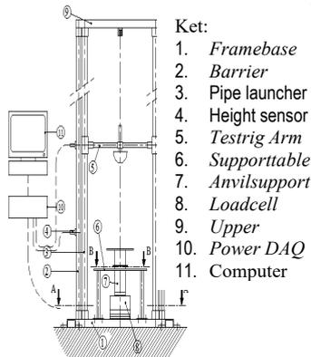
Figure 1: Free fall drop test impact
