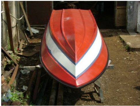
Figure 4: Fiber boat after gelcoat
