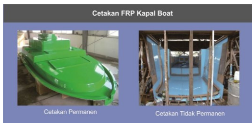
Figure 3: FRP mold permanent and non permanent.
