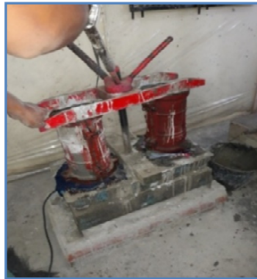
Figure 2. The compaction process uses a vibrating engine on all samples.
