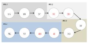
Figure 5 : Presedence diagram of recomendation work station.
