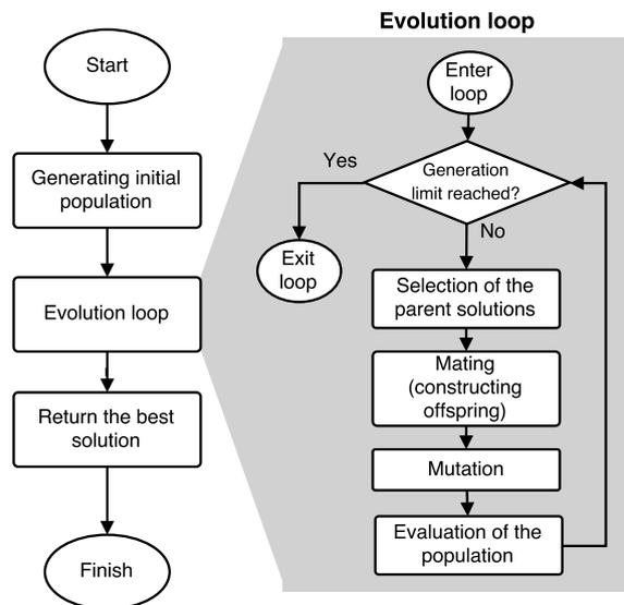
Figure 1: Flowchart of genetic programming with the evolution loop highlighted in the light gray background.
