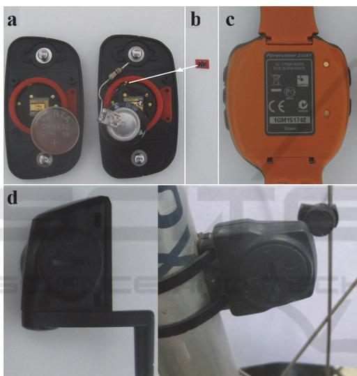
Figure 4: Collection of devices for discussion of charging concepts: a) backside mould of the open case of sensor S, and the installation of the SC plus required electronics b) voltage regulator IC installed left hand; c) commercial solution of contacting device for charging; d) pedal and wheel turning sensors as samples without regular contacts but battery mould.
