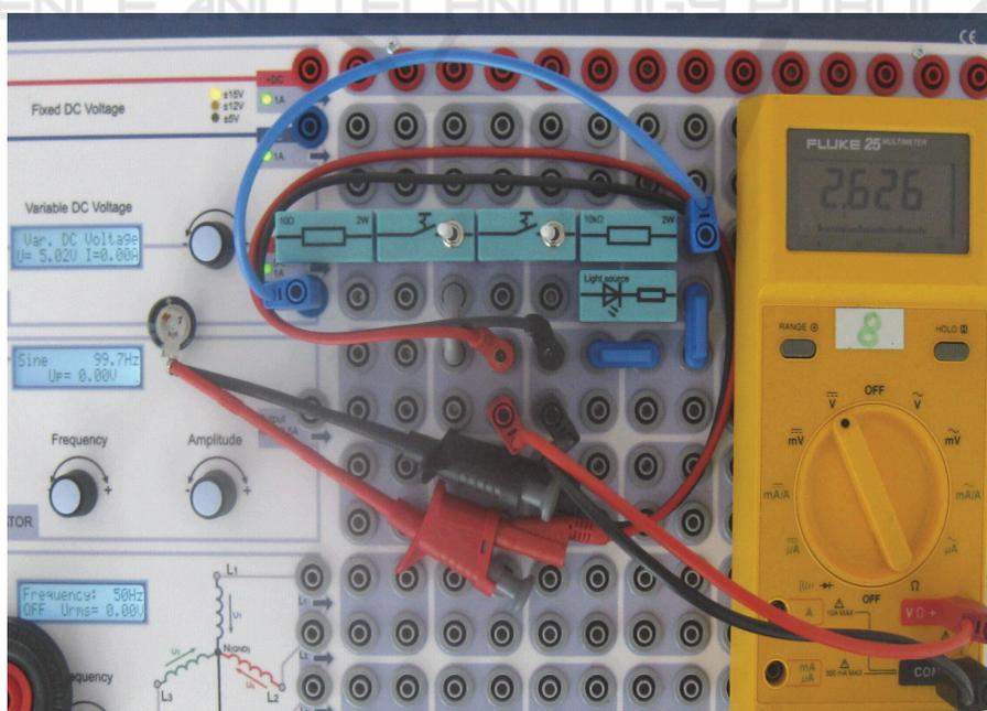
Figure 2: Laboratory board for charging and discharging the supercapacitor probe. A digital voltmeter measures precisely the probe output.
