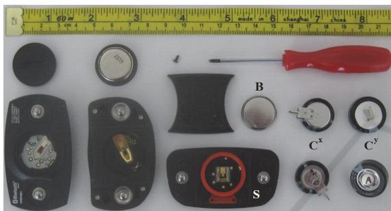
Figure 1: In here at bottom left, three different heart rate sensors are visible from backside. Above each sensor, its cover for the supply battery is shown, the middle one has to be fixed with four tiny screws. On bottom right, rear and top view of supercapacitors samples are shown, which are possibly feasible for replacing the lithium sensor batteries.
