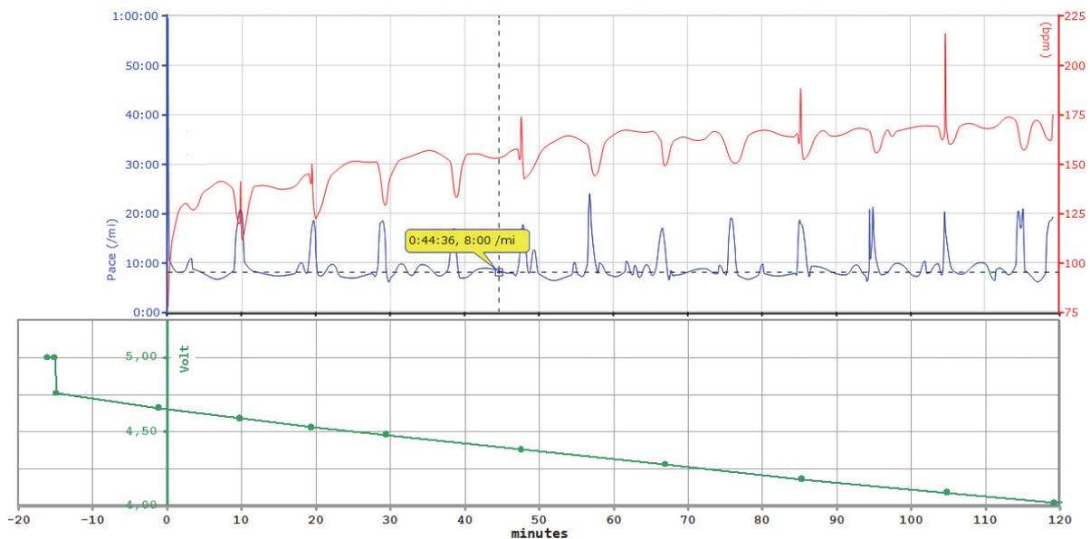
Figure 3: A half-marathon was covered by the run-walk-run method as reflected in the middle function plot, which displays the moving pace in units of minutes per mile. The lower curve shows the SC voltage, which was measured in the one minute walking breaks. This plot starts 15 minutes before the run with one minute charging at 5 Volts. The upper functional graph shows the HR curve, which suffers from distortion peaks induced by the voltage measurements.
