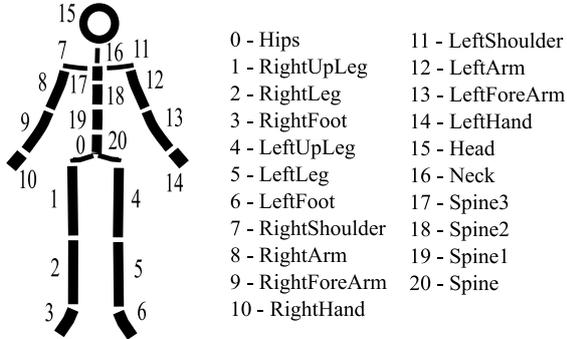
Figure 1: The structure of the skeleton estimated by the IMU-based system mocap along with the names of the segments.
