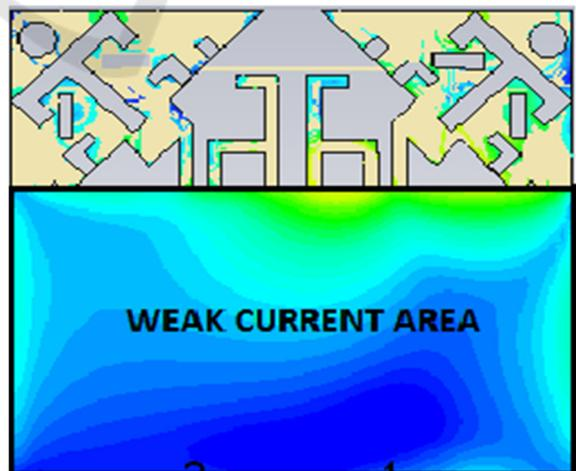
Figure 5: Current distribution on Ground for proposed ultra-wide band MIMO Antenna (colour slab is same as shown in Figure 3).
