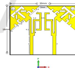
Figure 1a: Geometries of the Antenna.
