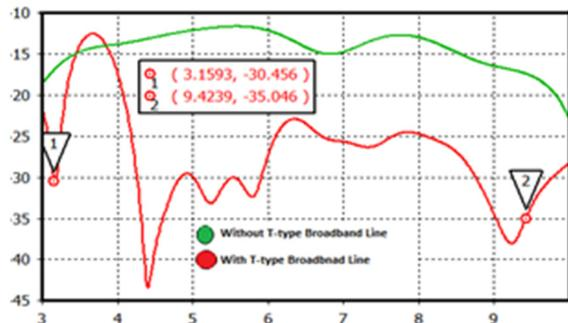
Figure 2: Simulated S-Parameters of ultra-wide band MIMO antenna comparing without T-type broadband line to with T-type broadband line.
