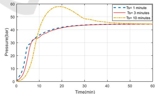
Figure 10: Effect of filter time constant on pressure loop.
