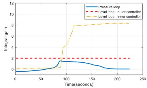
Figure 8: The PID coefficients profiles in adaptive control.
