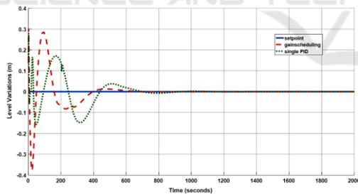
Figure 5: Gain-scheduled controller on drum variation level loop (desired value: zero variation).
