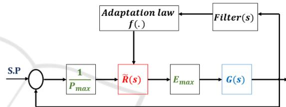
Figure 6: Self-tuning control scheme.
