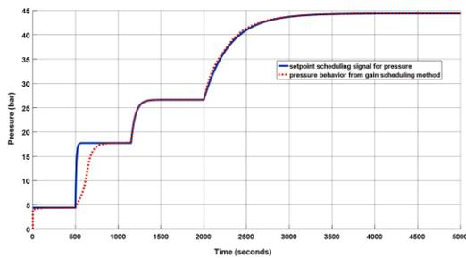
Figure 3: Drum pressure in different working points based on gain scheduled controller.
