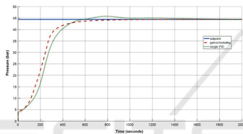
Figure 4: Gain-scheduled controller on drum pressure loop (desired value: 44.4bar).
