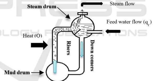
Figure 1: D-type water tube boiler.
