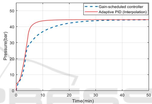
Figure 9: Comparison between self-tuning controller and gain-scheduled method.
