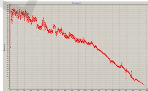
Figure 15: The graph of the altitude change depending on the frame number, the grid of points with the step of 50 pixels.
