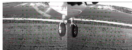
Figure 3: Points distributed along the regular grid on epipolar lines on the left frame and recalculated by the correlation to the right frame. The deviation of points from the epipolar on the right frame and the the epipolar deviation because of the lens distortion is notable.
