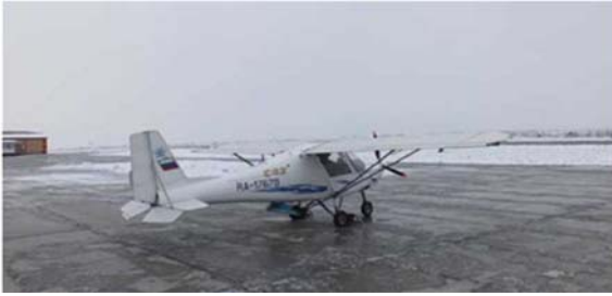
Figure 10: The Ikarus-C42 light plane onboard which the flying laboratory for studying of means of information support of aircrafts was organized.
