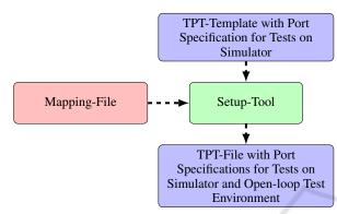
Figure 7: Data flow of the Setup-Tool for Creating Platform-independent TPT-Files.
