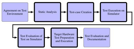
Figure 5: Proposed Workflow for Unit Testing.
