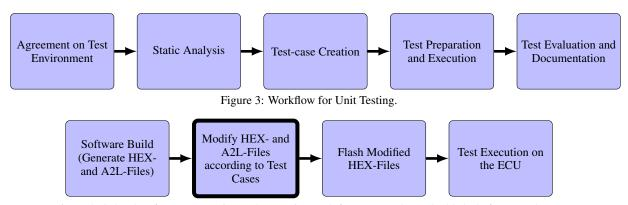
Figure 4: Subtasks of Test Preparation and Execution Task for Tests on the Embedded Platform Hardware.
