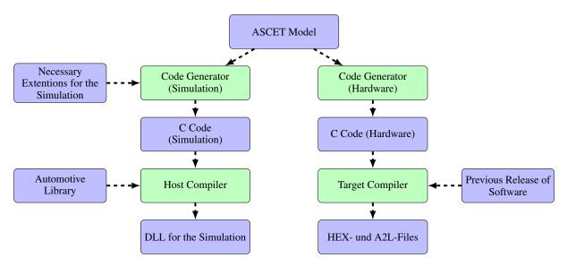
Figure 1: ASCET Code Generation for Simulation and Embedded Platform Hardware.
