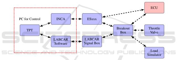
Figure 2: Open-loop Test Environment.
