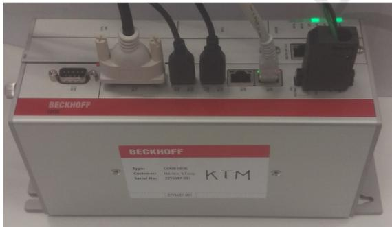
Figure 9: Industrial PC used for HiL validation.
