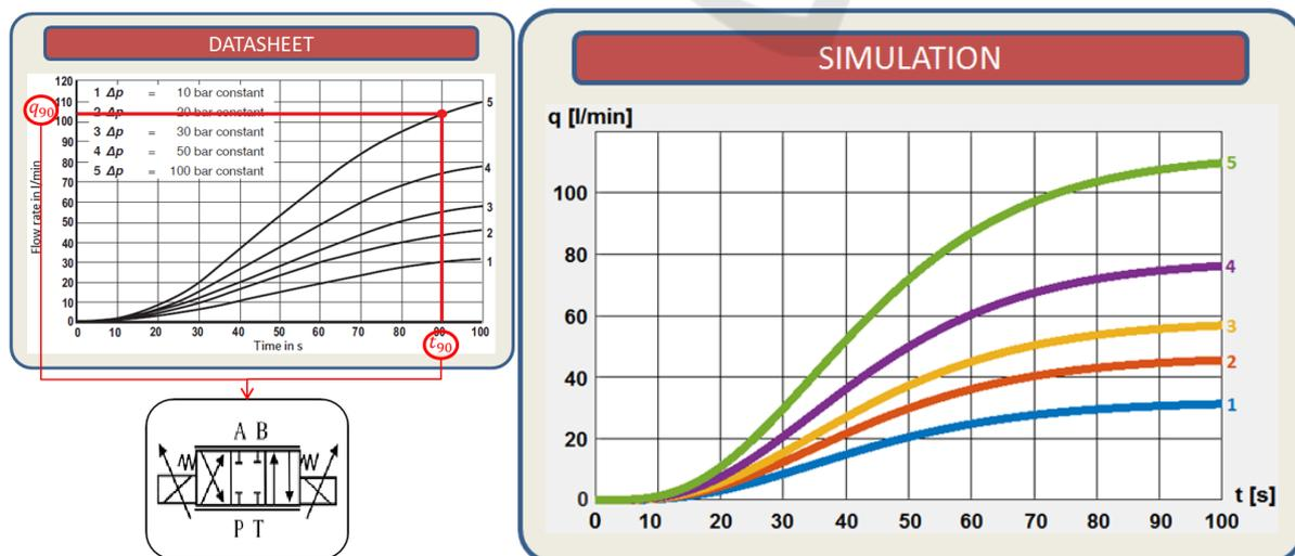
Figure 1: Proportional valve model configuration and simulation results.
