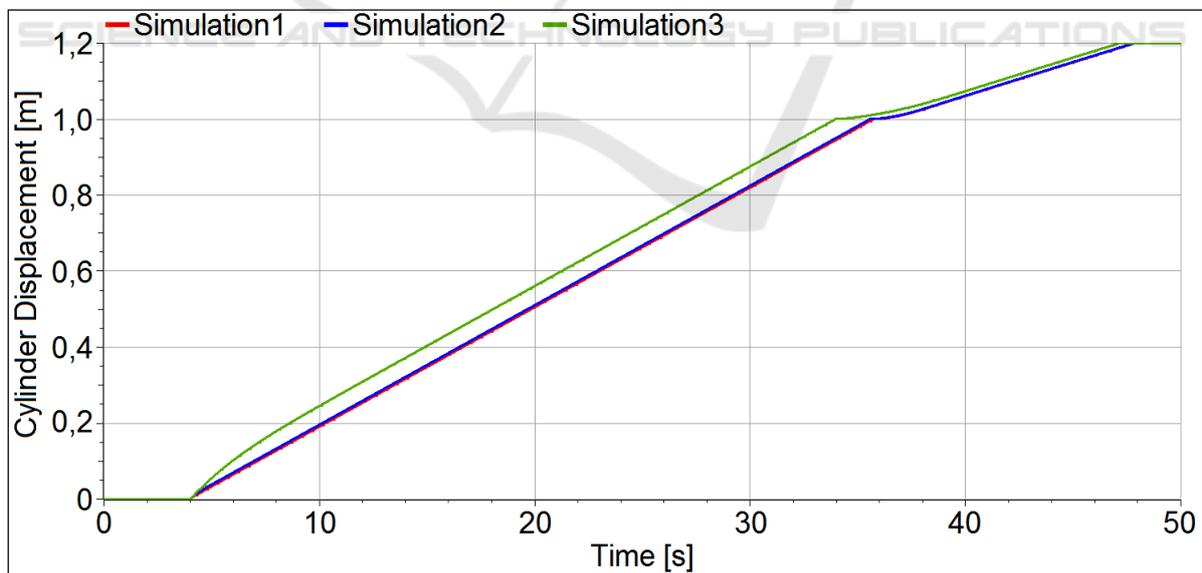
Figure 7: Cylinder displacement until contact is made with damper.
