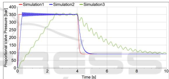
Figure 4: Proportional valve port P pressure.
