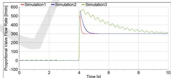
Figure 5: Proportional valve port P flow rate in litres per minute.
