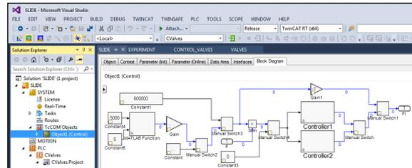
Figure 10: TcCOM Object with the controller developed in Simulink® and embedded in TwinCAT 3.
