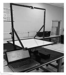
Figure 2: Experimental Ball and Plate System.
