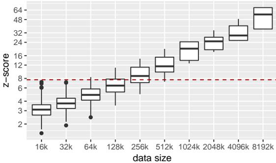
Figure 7: The size of the input bit stream vs.  $|Z\text{-score}|$  using distinguishers  $\{f_3, f_4, f_5, f_6\}$  for *Java Random*, 1000 random seed samples per data size category. Dashed line represents ref.  $Z\text{-score}$  value for the test.
