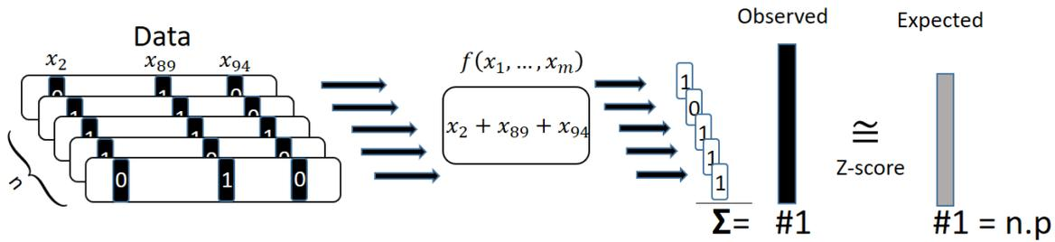
Figure 4: Our approach and the computation of  $Z\text{-score}$  using boolean function  $f(x_1, \dots, x_m) = x_2 + x_{89} + x_{94}$ .  $Z\text{-score}$  is computed as the statistical distance of observed #1 for tested data and  $\#1 = p.n$  expected for truly random data.
