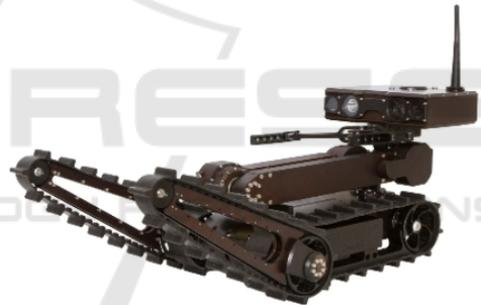
Figure 1: The Servosila "Engineer" crawler robot. Courtesy of Servosila company.
