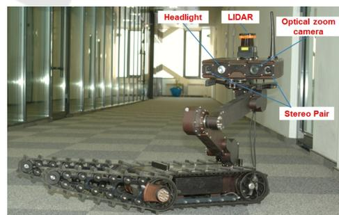
Figure 2: The "Engineer" robot head's sensor system.
