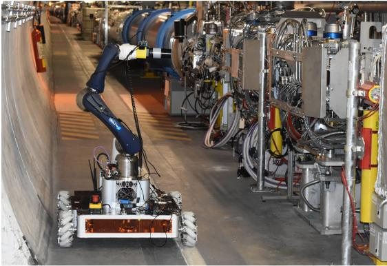
Figure 3: The robotic system used for this project during a test in front of a collimator of the LHC tunnel in Point 5.
