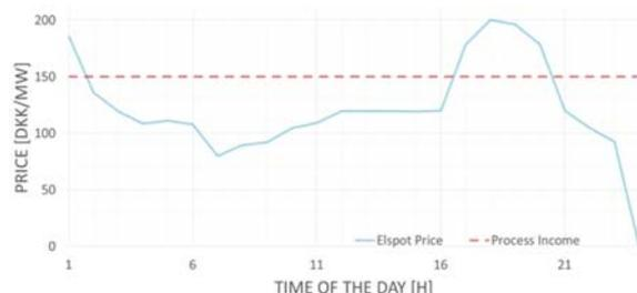
Figure 2: Example of the ON / OFF for the ideal process. The process is ON below the constant line.
