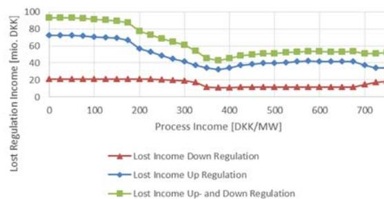
Figure 5: The lost regulation income of the 6 MW ideal process simulations for data from the DK-West Regulating Power Market.
