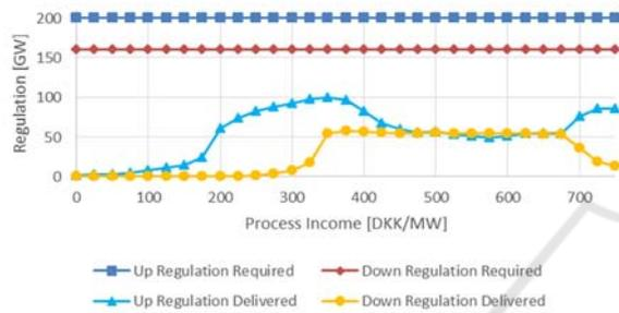
Figure 3: The flexibility potential of the 6 MW ideal process simulations for data from the DK-West Regulating Power Market.
