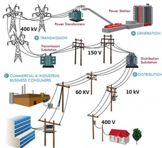
Figure 1: Overview of the Danish transmission and distribution grid (Clear Creek Networks, 2016).
