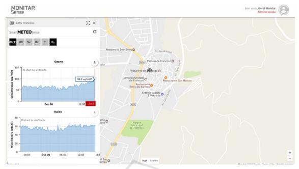
Figure 6: Display of web-based platform MONITAR SENSE showing ozone data and noise data from one of the MONITAR stations.
