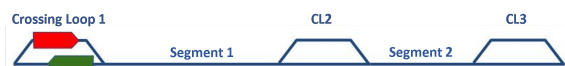
Figure 1: A Rail Transportation System with two single segments and three crossing loops.
