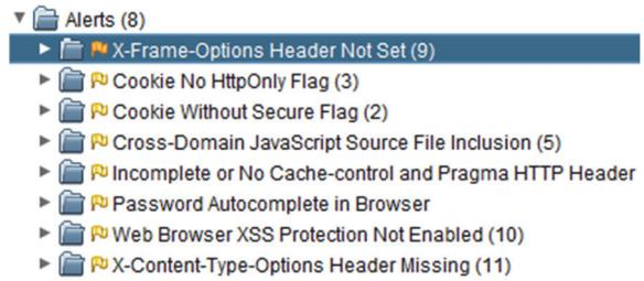
Figure 7b: ZAP Scan Result for Main Server (AWS) of Non-secure CDP.
