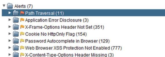
Figure 9b: ZAP Scan Result for CI Server (Jenkins) of Non-secure CDP.
