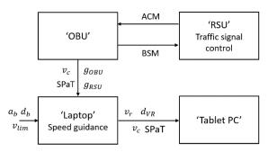
Figure 2: Flow chart of proposed eco-guidance system.
