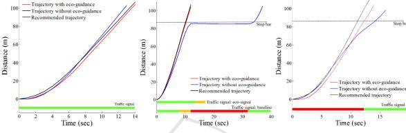
Figure 7: Time-moving distance graph in scenario 1.
