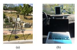
Figure 1: Devices for a field test; (a): RSU; (b): Laptop, tablet PC, and OBU.
