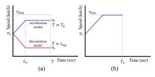
Figure 5: Acceleration/deceleration profile; (a): acceleration /deceleration to the recommended speed; (b): acceleration to the speed limit.
