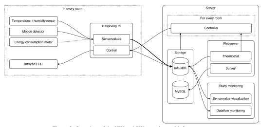
Figure 3: Overview of the HW and SW experimental infrastructure. Table 1: Average power consumption over all rooms B and C only and over each room separately.
