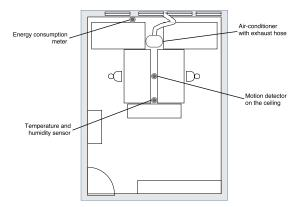
Figure 2: Sensor and actuator deployment.
