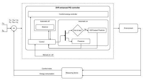
Figure 1: SVReCLCE control loop and its elements.
