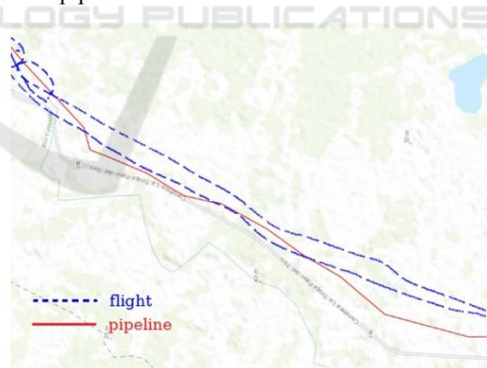
Figure 3: Inaccurate flight without pipeline tracking.
