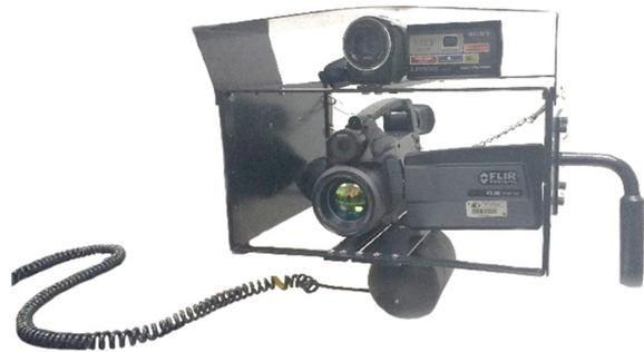
Figure 2: IR and HD video cameras recording frame.
