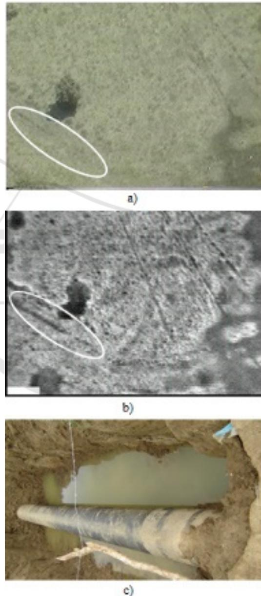
Figure 17: Place that was determined as pipeline with severe problems (loss of insulation covering) by means of aerial inspection and intelligent "pig". a) HD screenshot b) IR screenshot c) Verification photograph.
