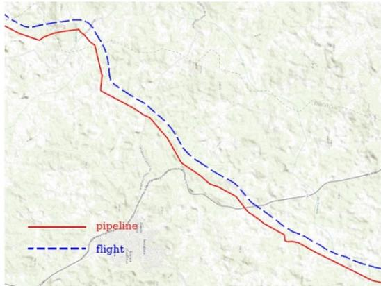
Figure 4: Flight with pipeline tracking.
