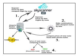
Figure 4: Architecture diagram.
