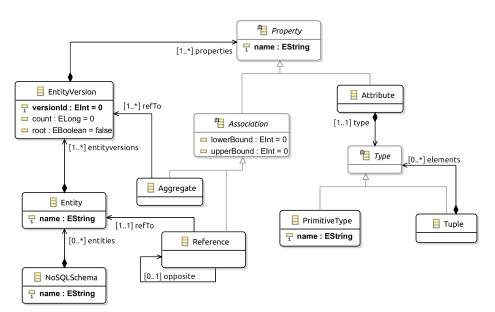
Figure 1: NoSQL Schema Metamodel.
